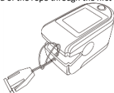
Figure 4. Mounting the hanging rope.
